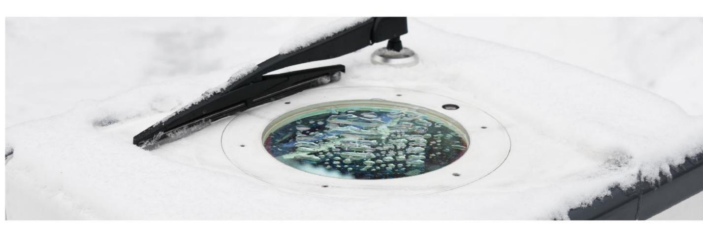
The Molas B300 wind measurement lidar uses the laser Doppler effect and uses the four-beam VAD scanning vector synthesis technology to complete the measurement of wind speed and wind direction at 30-300 meters above the lidar. it can be fully equivalent to a wind tower with a height of 300 meters.
