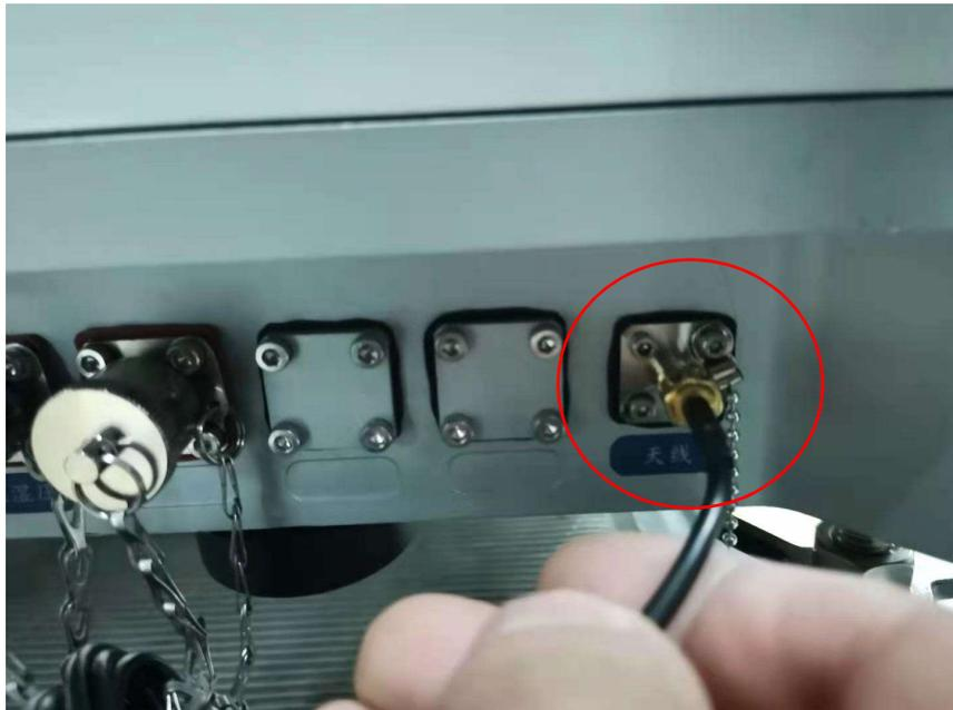
Figure 12 Installing the antenna
