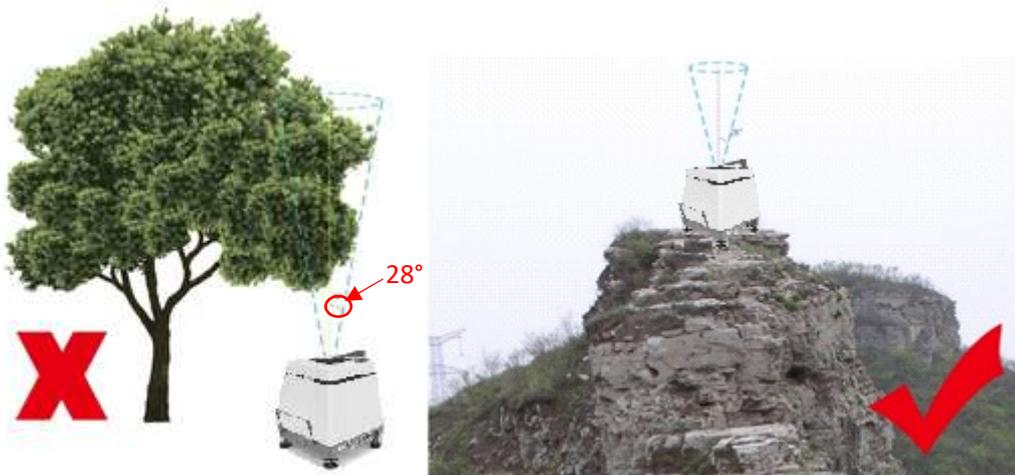
Figure 5 Lidar Installation Location Diagram
